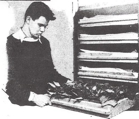
Top, Throwing Stones into Mill to Grind Up Dried Leaves and Extract the Chlorophyll; Center, Some Pure Chlorophyll; Right, Drying the Green Leaves
